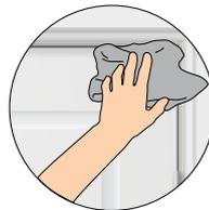
**1 CLEANING SURFACES** - Clean the door and door jamb to be weather stripped. For best results, weather stripping should be applied to clean, dry surfaces above 20°F.
