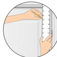
**2 MEASURING DOOR & DOOR JAMBS** - To ensure greater accuracy, measure your space twice before cutting the material. It is best to plan for one continuous strip for each side of the door and door jamb.
