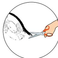
**3 CUTTING FOAM** - Cut long pieces of self-adhesive weather stripping material (foam, vinyl, etc.) for each side of the door jamb and door.
